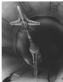
Fig. 10 0.08-scale F/A-18E model in the Langley 16-ft Transonic Tunnel.
