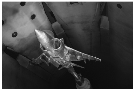
Fig. 23 0.15-scale AV-8B model mounted on the FTR rig in Langley 16-ft TT.
