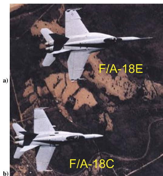
Fig. 2 Photo of the a) F/A-18E and b) F/A-18C in flight. Note snag on E leading edge.
