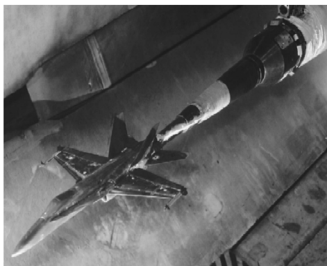
Fig. 25 0.06-scale F/A-18C model mounted on the FTR rig in Langley 16-ft TT.
